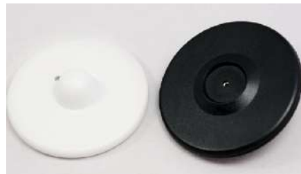
Large Round No.T002 Frequency: 8.2MHz/1.95MHz/3.25MHz/4.75MHz Dimension: Ø58mm Color: Black/White or Customized Lock: Standard/Super Packing: 38x31x19.5cm, 500pcs/ctn, 6.3kgs/ctn
